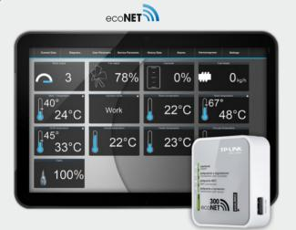
An ecoNET 300 internet module ensures remote access to the controller using PC, tablet or mobile phone. The user has the ability to edit basic and service parameters thus having an inluence upon operation of heat recovery unit. From the user point of view, a clear and straightforward interpretation of operational history in form of graphs is an additional advantage.
